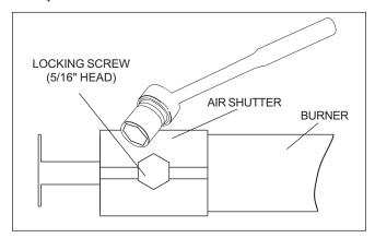
Figure 13. Air Shutter Adjustment.
